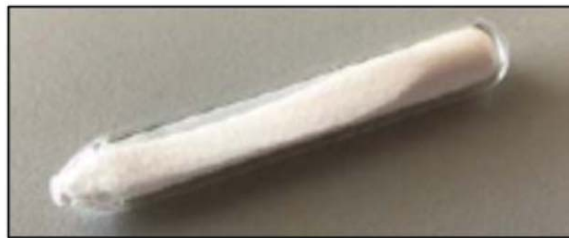
Figure 1: Target Ampule – Cylindrical fused quartz body containing target material
