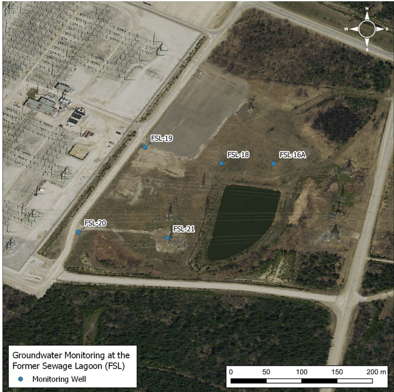
Figure 46 Shallow Groundwater Monitoring Well Locations - FSL
