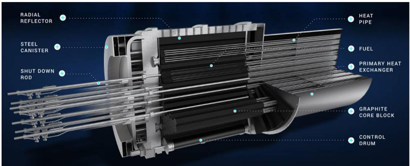
fig. 2 eVinci micro reactor containers
