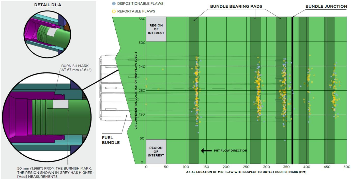
NO FLAWS in the limited region of interest where hydrogen concentration is above model predictions (<0.5% of tube)
