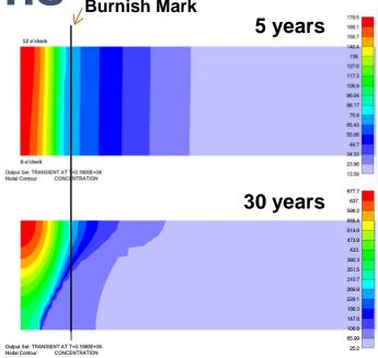
Higher than predicted hydrogen concentrations are limited to a localized (<0.5%) volume in the upper portion of the pressure tube.
