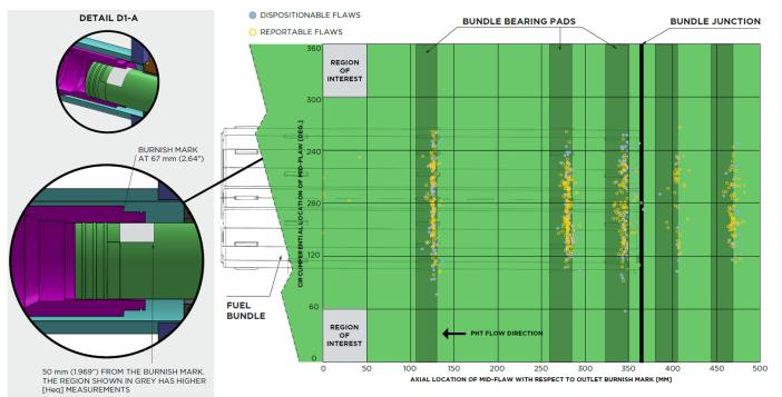
NO FLAWS in the limited region of interest where hydrogen concentration is above model predictions (<0.5% of tube)
