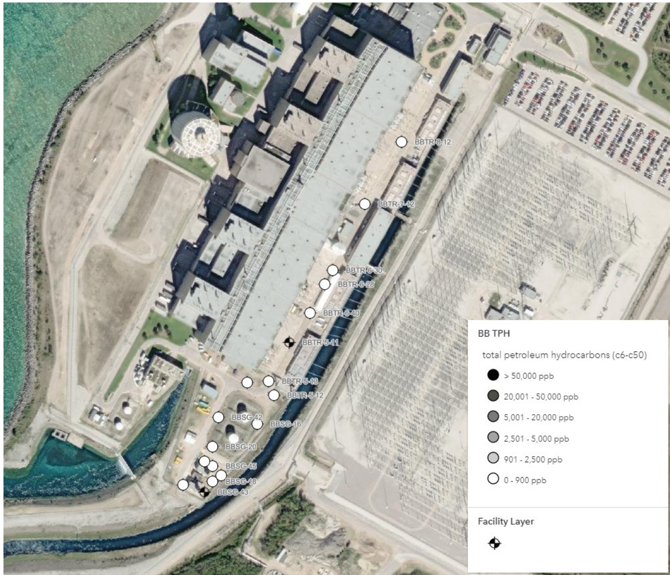
Figure 68 - Aerial Map of the Bruce B Transformer Area and the Bruce B Standby Generator Area (Bruce B Area) with Monitoring Well Locations Shaded According to Concentration Range of Total Petroleum Hydrocarbons
