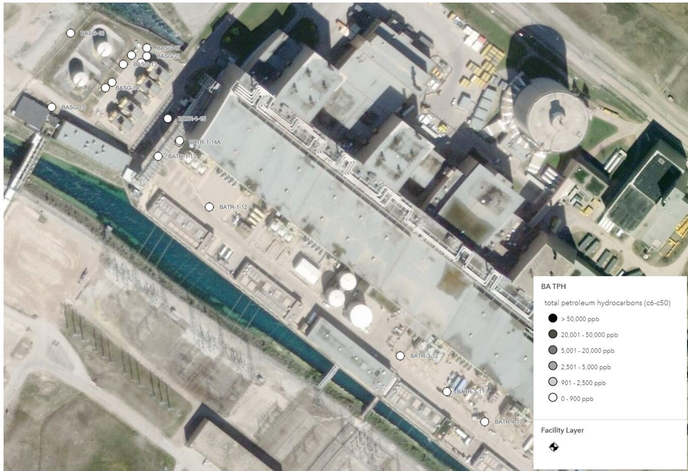
Figure 67 - Aerial Map of the Bruce A Transformer Area and the Bruce A Standby Generator Area (Bruce A Area or Area 1 of Figure 1) with Monitoring Well Locations Shaded According to Concentration Range of Total Petroleum Hydrocarbons
