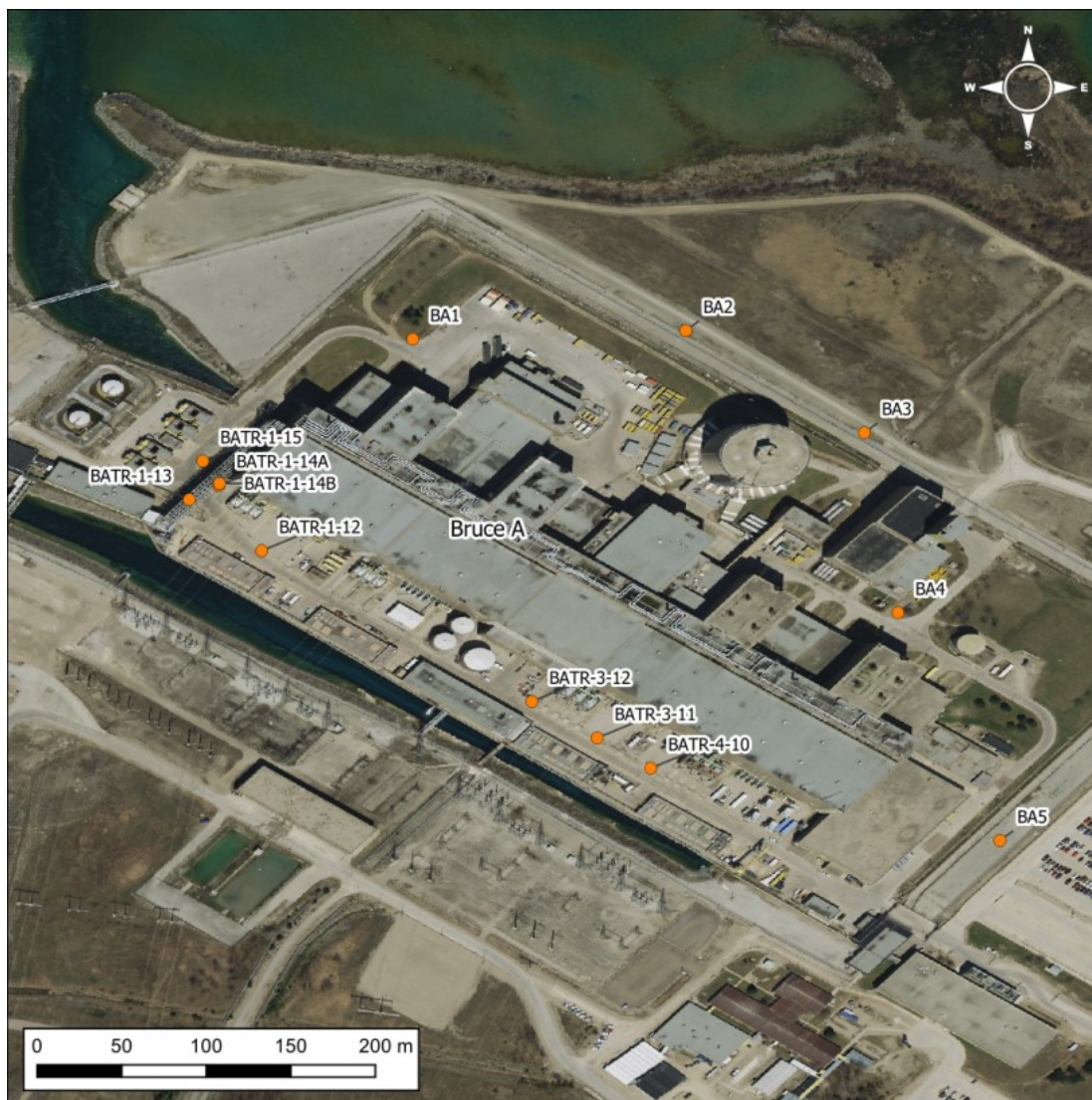
Figure 59 - Groundwater Monitoring Well Locations Sampled for Tritium at Bruce A
