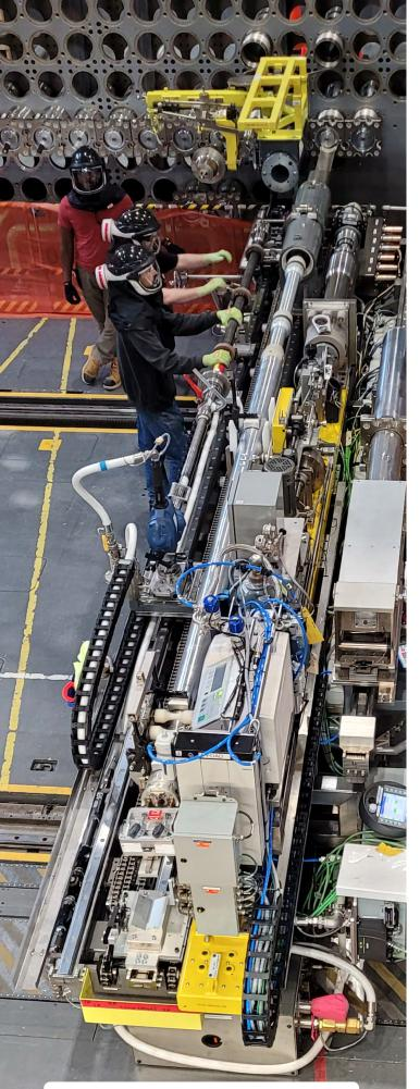
Multi-Purpose Installation Worktable (MIWT) and Vision Alignment System (VAS) Calibration Fixture:
