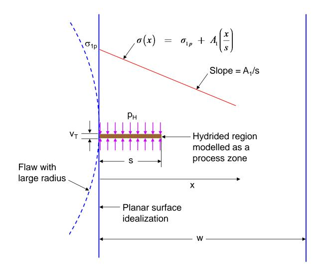
Figure A-1: Process Zone Emanating from a Planar Surface and Subjected to an Applied Linear Stress Distribution
