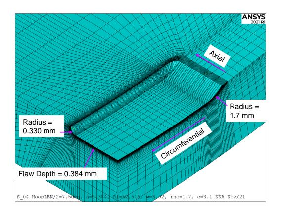
Figure 6-2: View of CWEST Scrape Flaw in Bruce Unit 3 for the Baseline Case B3-1 with a Flaw Depth of 0.384 mm and a Corner Root Radius of 1.7 mm in the Three-Dimensional One-Quarter Symmetry Finite Element Model
