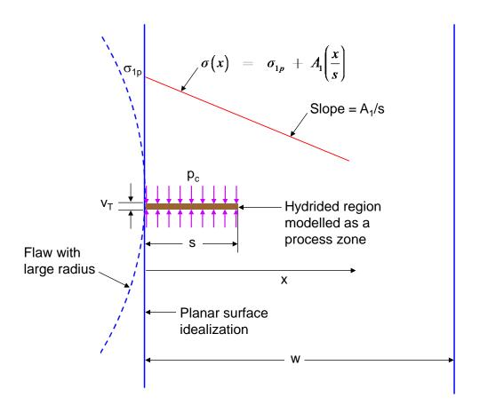
Figure 7-1: Process Zone Emanating from a Planar Surface and Subjected to an Applied Linear Stress Distribution
