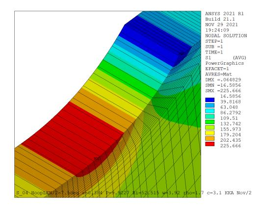
Figure 6-4: Close-Up View of Maximum Principal Stress Contours at CWEST Scrape Flaw in Bruce Unit 3 for the Baseline Case B3-1 with a Flaw Depth of 0.384 mm, a Corner Root Radius of 1.7 mm, and a Total Nominal Hoop Stress During Hydride Precipitation of 142.9 MPa Including Pressure on the Flaw Face
