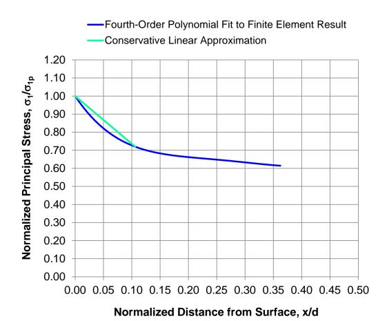
Figure A-3: Illustration of the Conservative Linear Stress Distribution
