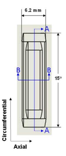
Figure 3-2: Top View of CWEST Scrape Flaw
