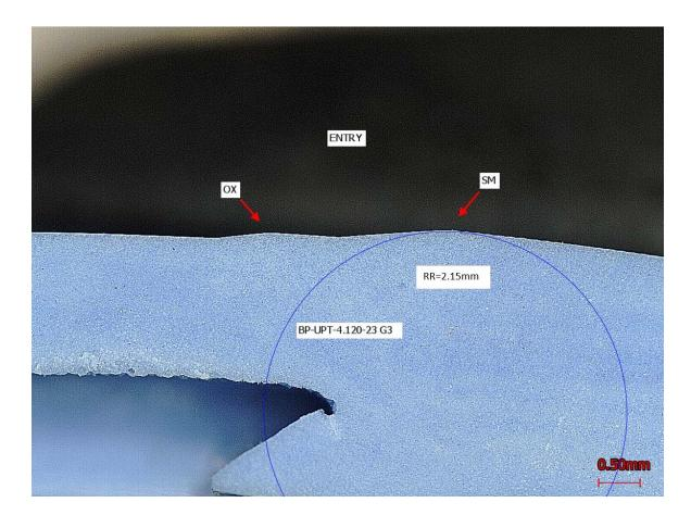
OX: Oxide cut SM: Sample cut RR: Root radius
