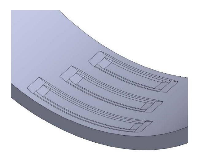
Figure 3-1: Illustration of CWEST Scrape Flaws
