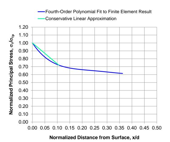
Figure 7-2: Illustration of the Conservative Linear Stress Distribution
