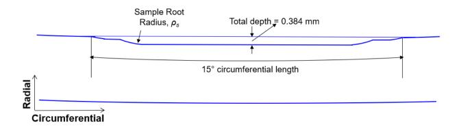
Figure 3-3: CWEST Scrape Flaw Geometry in the Radial-Circumferential Plane of the Pressure Tube (Section A-A of Figure 3-2)
