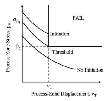
Figure A-2: Various  $p_H$  Versus  $v_T$  Behaviour as a Hydrided Region Develops at a Flaw Tip Illustrating the Threshold Peak Stress for DHC Initiation,  $\sigma_{th}$
