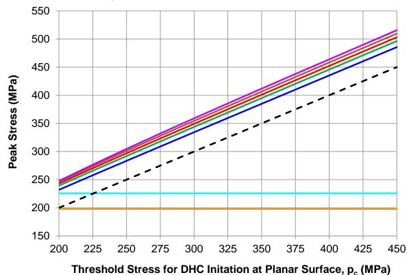
Figure 8-2: Variation of Predicted Threshold Peak Stress for DHC Initiation,  $\sigma_{th}$ , with  $p_c$  for a Range of  $K_{IH}$  for Bruce Unit 3 Baseline Case B3-1, and Bruce Unit 7 Baseline Case B7-1, with a Scrape Flaw Depth of 0.384 mm and a Corner Root Radius of 1.7 mm, with the Applied Peak Stresses
