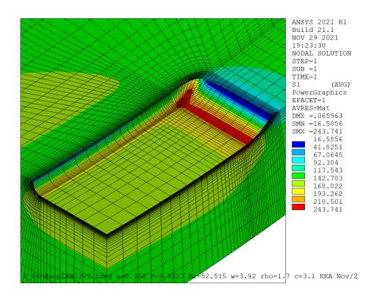
Figure 6-3: Maximum Principal Stress Contours at CWEST Scrape Flaw in Bruce Unit 3 for the Baseline Case B3-1 with a Flaw Depth of 0.384 mm, a Corner Root Radius of 1.7 mm, and a Total Nominal Hoop Stress During Hydride Precipitation of 142.9 MPa Including Pressure on the Flaw Face
