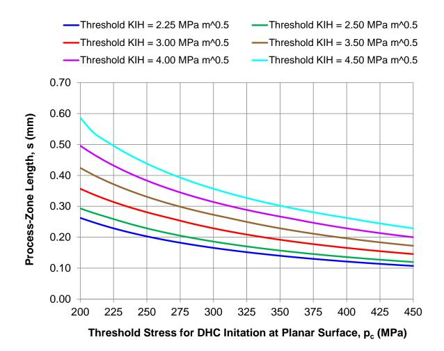
Figure 8-1: Variation of Predicted Process-Zone Length, s, with  $p_c$  for a Range of  $K_{IH}$  for Bruce Unit 3 Baseline Case B3-1 with a Scrape Flaw Depth of 0.384 mm and a Corner Root Radius of 1.7 mm
