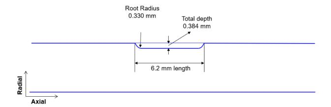
Figure 3-5: CWEST Scrape Flaw Geometry in the Radial-Axial Plane of the Pressure Tube (Section B-B of Figure 3-2)
