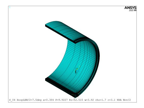
Figure 6-1: Three-Dimensional One-Quarter Symmetry Finite Element Model of Pressure Tube with the CWEST Scrape Flaw in Bruce Unit 3 for the Baseline Case B3-1 with a Flaw Depth of 0.384 mm and a Corner Root Radius of 1.7 mm
